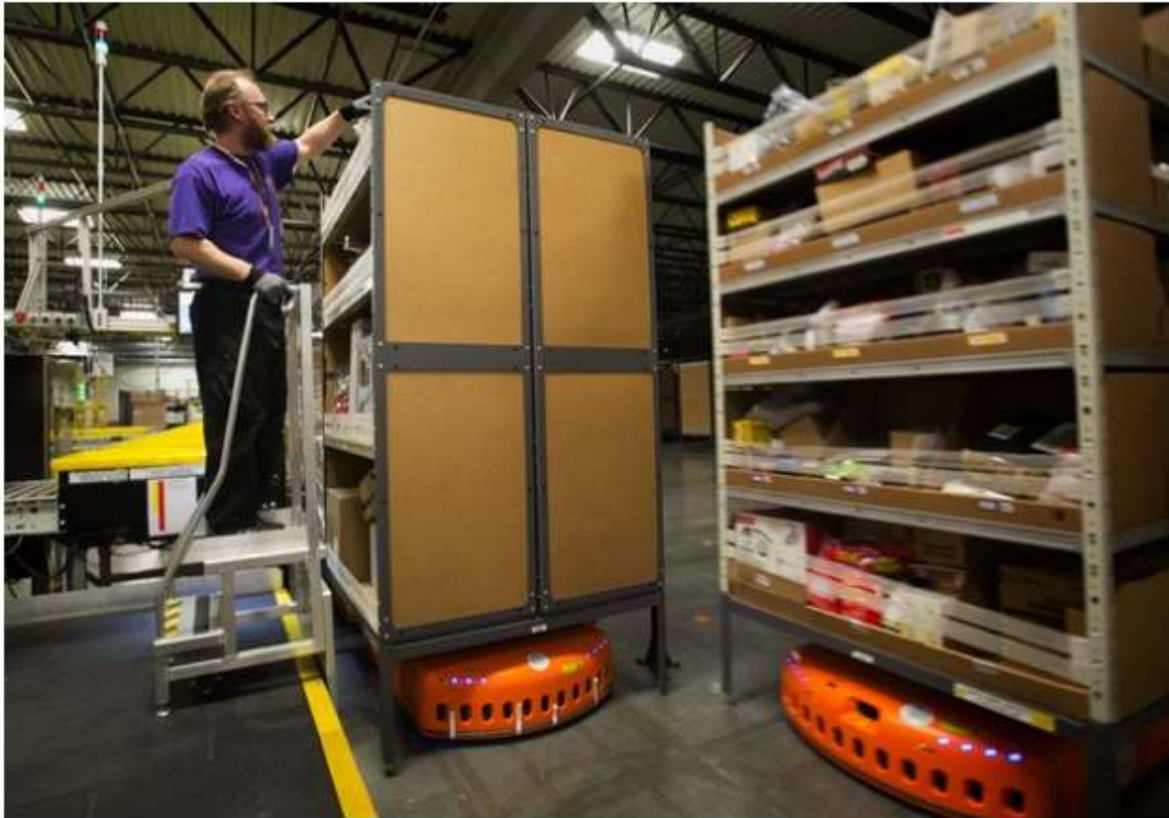
An Amazon worker removes packages from a container on top of a Kiva robot. (Ellen M. Banner/The Seattle Times)
